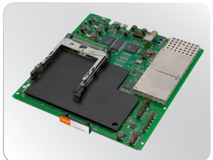
Quad COFDM backend module - with 2 x CI slots
